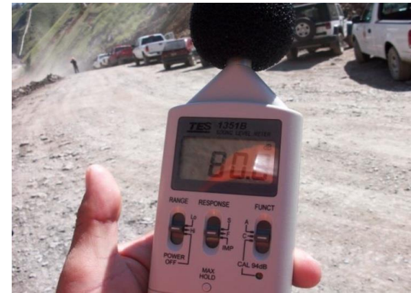
Figure 48 (left) Sound monitoring in front of a tunnel. Figure 49 (right). Sound monitoring of a terracing site. Source: CONNET. Monitoreo de Ruido . Photo report, n.d.
