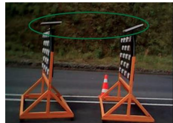
Figure 50 (left) and Figure 51 (right). Solar powered signs and lights are used for highway operations. Source: CONNET. Señalamiento Solar . Photo report, n.d.
