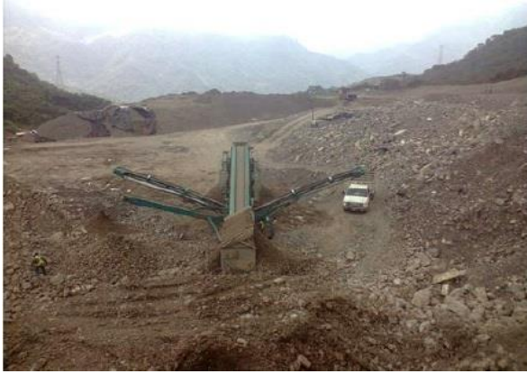
Figure 58 (left) and Figure 59 (right). A gravel crusher uses the extracted rock material to be reused in the project. Source: CONNET. Planta Trituradora . Photo report, n.d.
