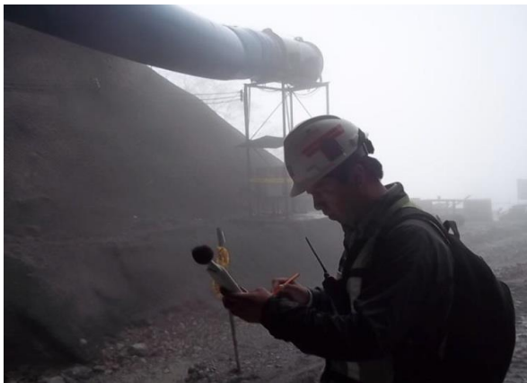
Figure 48 (left) Sound monitoring in front of a tunnel. Figure 49 (right). Sound monitoring of a terracing site. Source: CONNET. Monitoreo de Ruido . Photo report, n.d.
