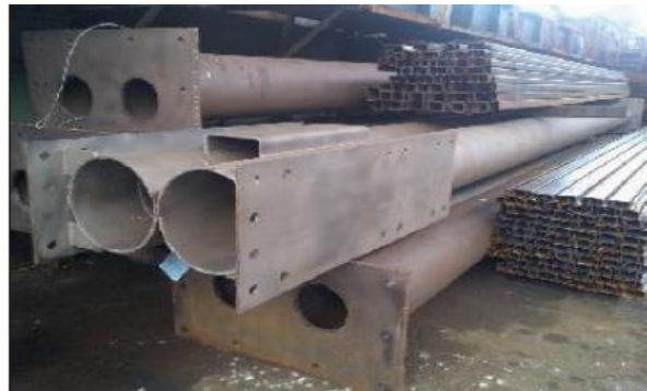
Figure 52 and 53 : Materials and resources. LEED L-20.2 MR-5.1; MR-5.2. Reuse of material from the old terminal.
