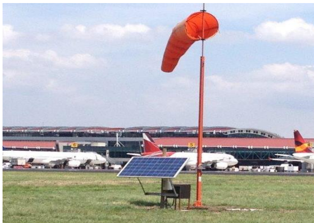
Figure 33: Use of solar energy to provide power to the meteorological station. Source: Picture provided by AERIS April 2013
