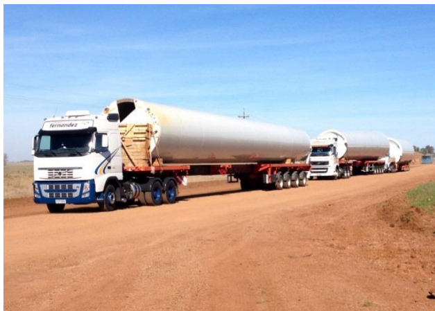
Figure 13: Trucks transporting the pre-fabricated towers to the site, during construction process. Source: Picture taken during the onsite visit May 2013
