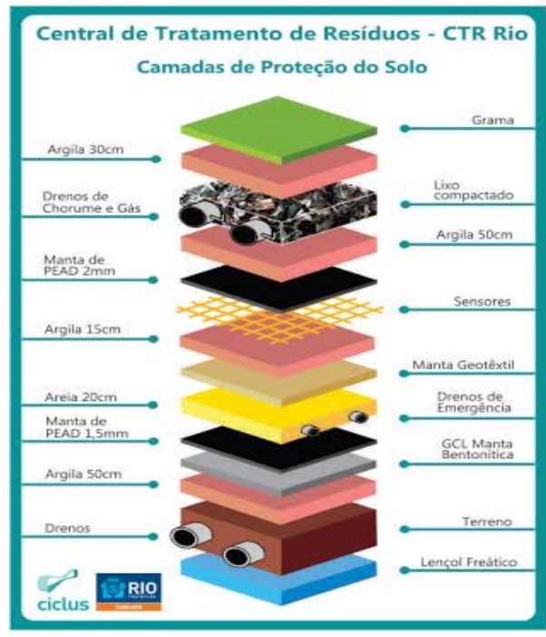
Figure 20: Waterproofing system implemented in CTR Rio. Sources: Ciclus. Accessed in 2015 http://www.ciclusambiental.com.br/ciclus_ctr.php
