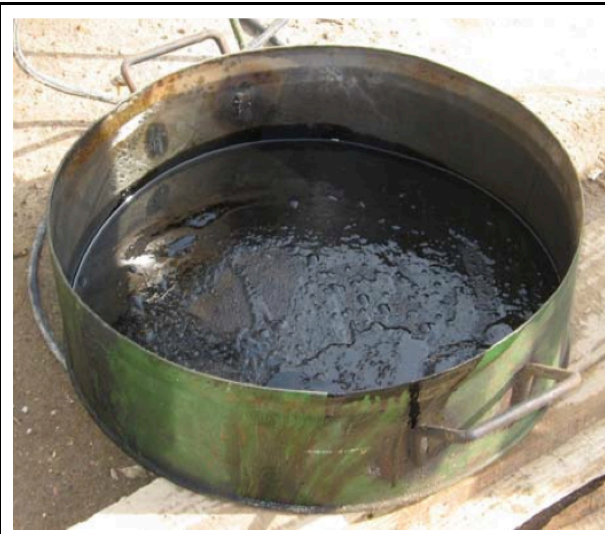
Figure 19: Fluids contained to be filtered and disposed in specific containers meant for each filtered liquid. Sources: CSI Ingenieros, Plan Gestión Ambiental Etapa de Construcción (PGA), Abril 2012, p. 41.
