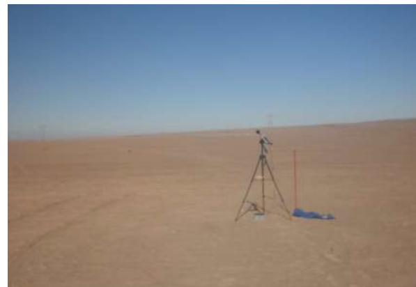
Figure 11: Noise monitoring station Sources: Corporación de laboratorios ambientales del peru S.A.C. , Air quality and ambient noise monitoring, preliminary evaluation of solar photovoltaic plant Moquegua (Peru, 2012), 25
