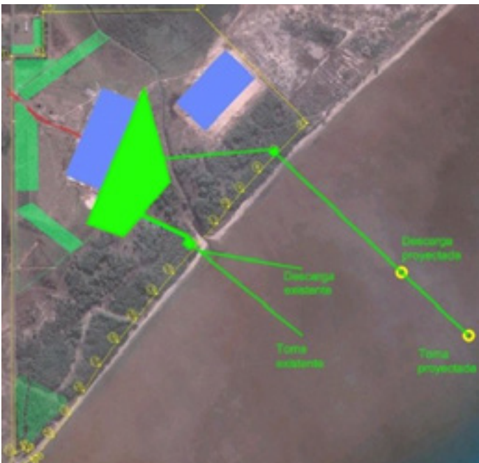
Figure 5: Points of water intakes and effluent discharges of the cooling system of the existing (PTA) and new (PTB) power plants within the Santa Lucia wetland area.
