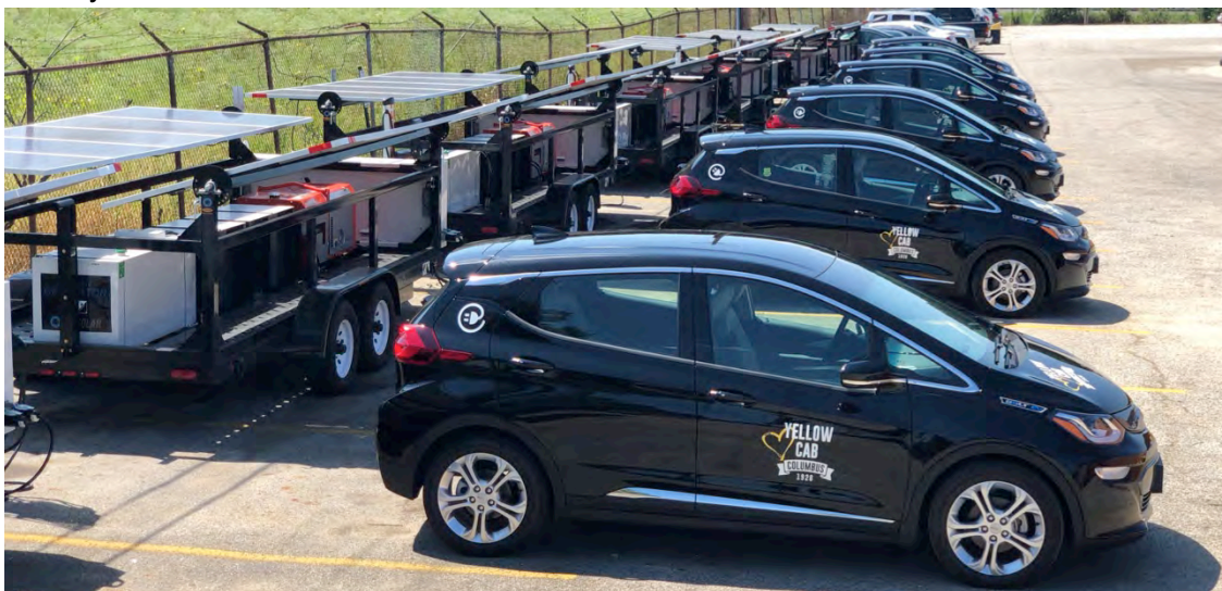
Figure 11. CYC EVs and DC Solar charging units. Source: CYC, 2018.
