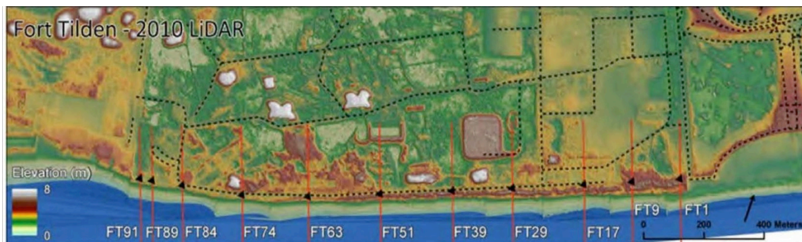
Digital Elevation Model of Shore Road area within Fort Tilden prior to Hurricane Sandy, derived from 2010 LiDAR data. Light green elevations are in the flat sandy beach. Dark green elevations are in the upper beach adjacent to the dune and inland of the dune feature. Tan and brown elevations are higher than the sand beach, they characterize the dune feature. Shore Road is the dotted line immediately inland of the beach. Other dotted lines represent locations of existing roads identified on orthophotos. In addition, the figure includes the locations of profile lines that were constructed using LiDAR data sets (from 2010 and from 2012) and field surveys conducted in December, 2014.
