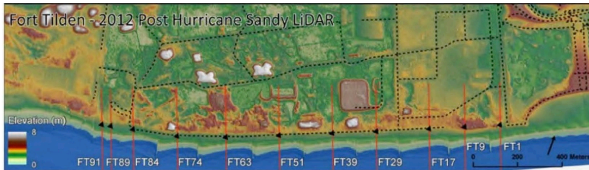
Digital Elevation Model of Shore Road area within Fort Tilden after Hurricane Sandy, using post-Sandy 2012 LiDAR data sets. Elevation categories are the same as in Figure 1. Dotted lines represent locations of roads prior to Hurricane Sandy. Black triangles on profile line locations represent the 0.0 distance position incorporated on the profiles. The profiles extend seaward and landward from these starting points
